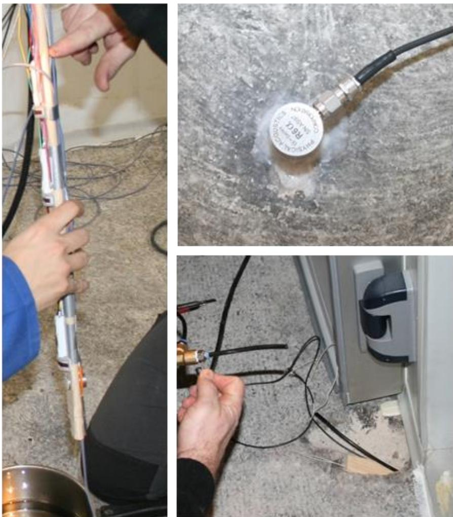
Fig. 4. Location of the ultrasonic sensors on a plane view (top) and vertical view (bottom).
