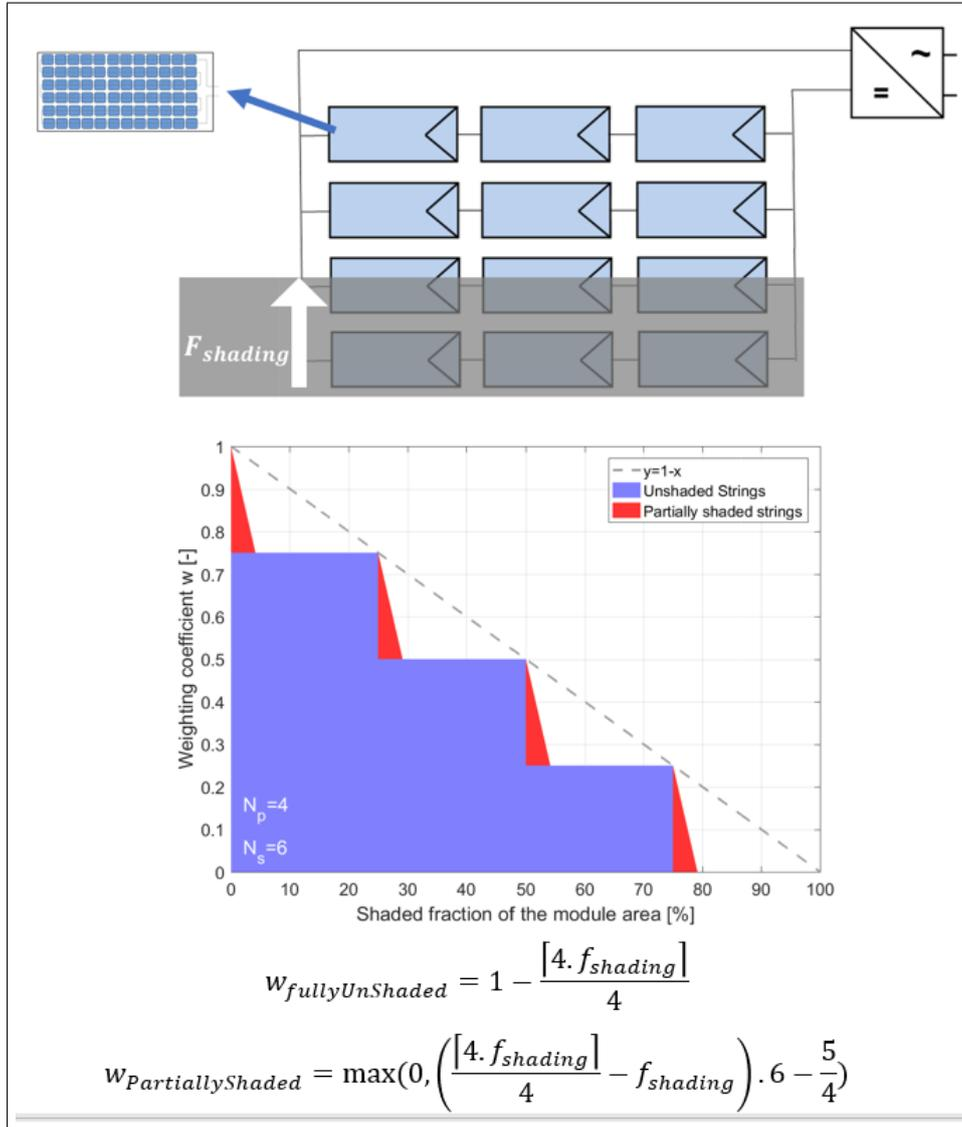
Figure 17: Example of  $N_s$  and  $N_p$ ,  $w_{FullyShaded}$  and  $w_{PartiallyShaded}$  computation for a row of 6x12-cells panels in landscape orientation. The panel connection are 3 in series and 4 in parallel.
