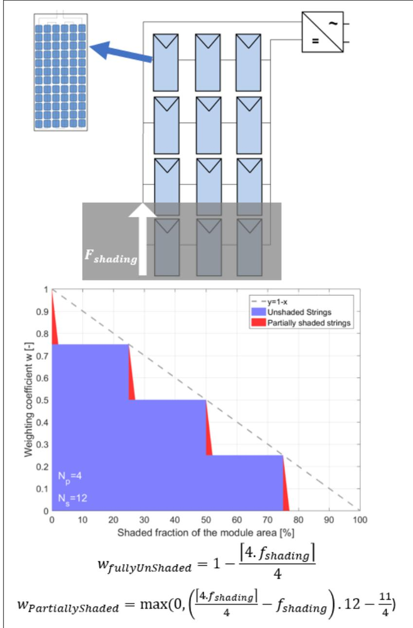
Figure 19: Example of  $N_s$  and  $N_p$ ,  $w_{FullyShaded}$  and  $w_{PartiallyShaded}$  computation for a row of 6x12-cells panels in portrait orientation. The panel connection are 3 in series and 4 in parallel.
