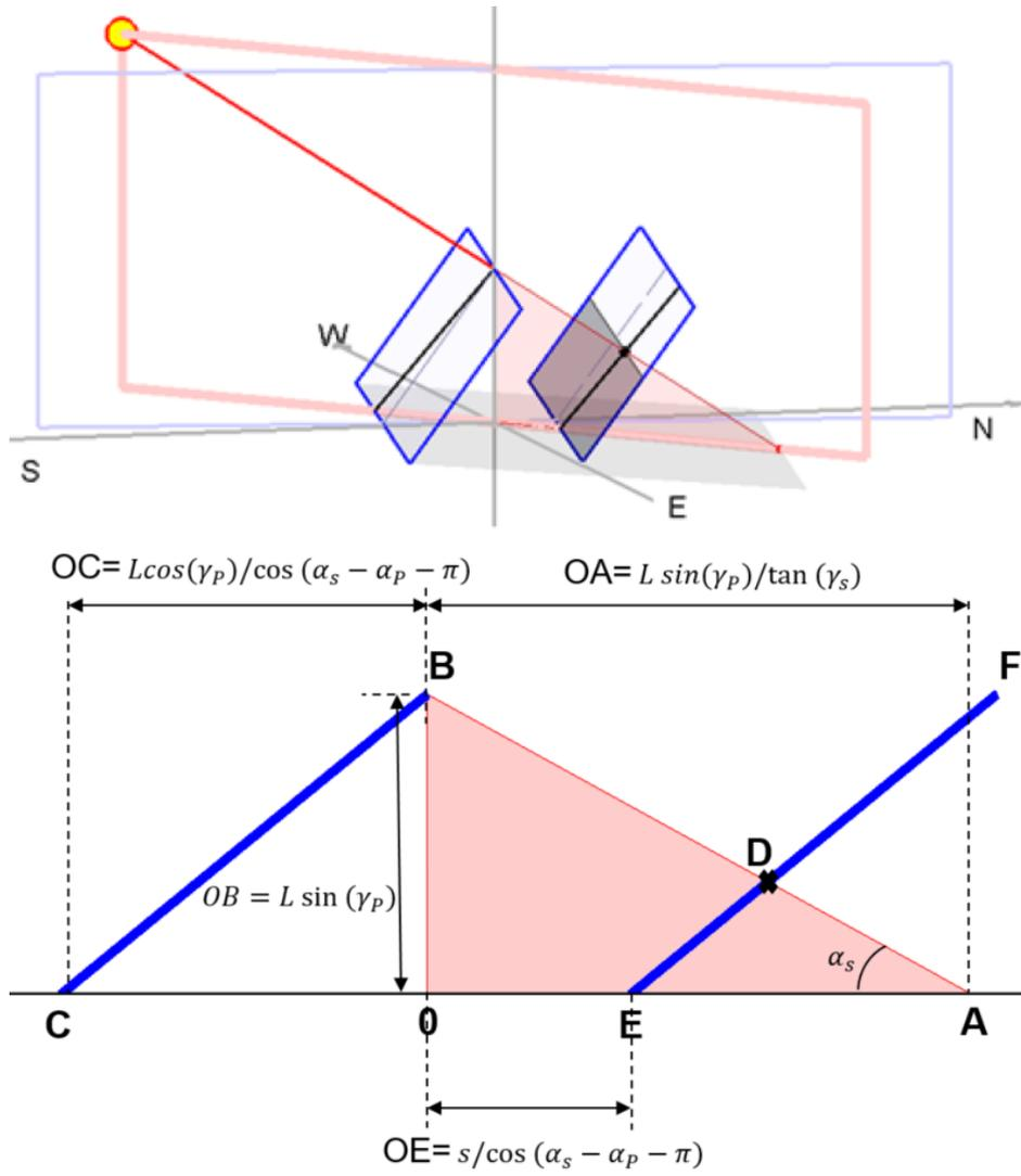
**B Example of  $N_s$  and  $N_p$ ,  $w_{FullyShaded}$  and  $w_{PartiallyShaded}$  computation**
