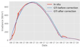
Figure 6: Comparison with -35° tilted reference cell and satellite-derived GTI before and after correction
