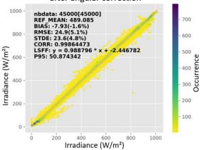
**Figure 5:** All sensors measurements in the 6 lastmonths 2017 period in clear sky days vs GTI from McClear model, with corrected tilt and azimuth angles. Correction was done in the first 6-month 2017 period.
