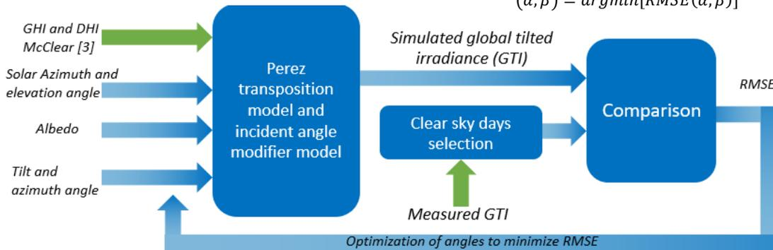
**Figure 1:** Illustration of the different steps of the software correction method for angle misalignments
