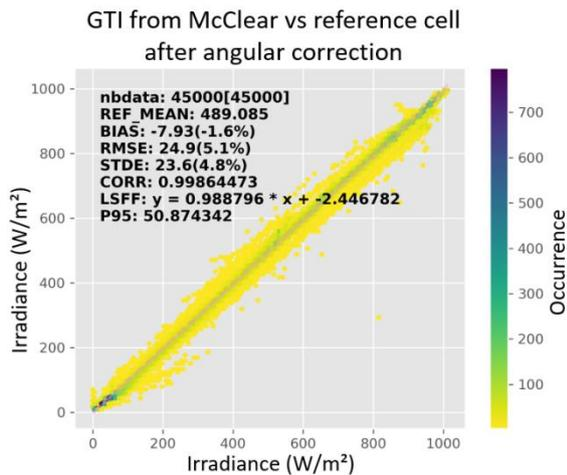
**Figure 5:** All sensors measurements in the 6 last-months 2017 period in clear sky days vs GTI from McClear model, with corrected tilt and azimuth angles. Correction was done in the first 6-month 2017 period.
