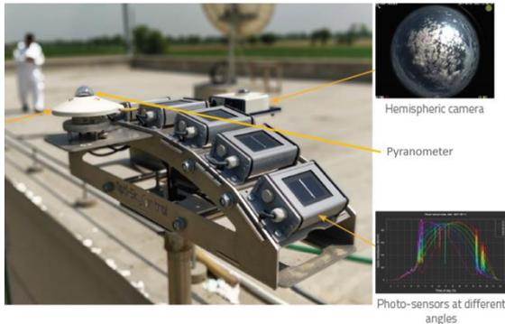
**Figure 2:** Opti-SkyControl© Sensors developed by Optimum Tracker company
