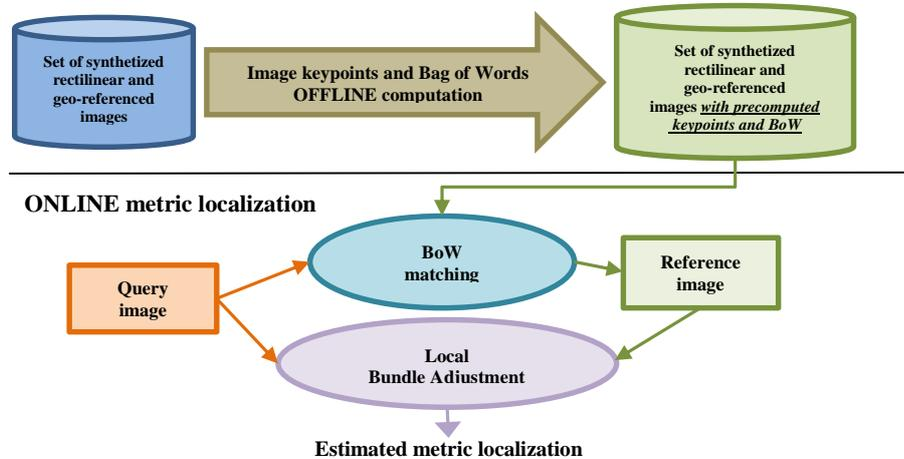
**Fig. 4.** Pipelines for our method 1: on top, keypoints and BoW are pre-computed *offline* on all synthesized geo-referenced images; on bottom, the 2 steps for online metric localization.
