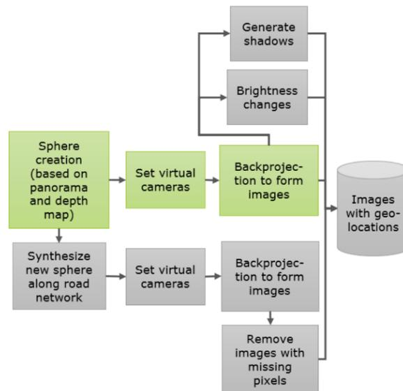
**Fig. 1.** Pipeline for offline generation of geo-referenced rectilinear images from each StreetView panorama.
