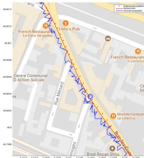
**Fig. 7.** Example of estimated positions with our pose regression CNN approach (blue line), to be compared with the ground truth trajectory (red line). The red dots are the positions of pre-existing StreetView panoramas.
