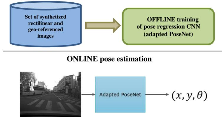
**Fig. 5.** Pipelines for our method 2: on top, a pose regression CNN is pre-trained *offline* on the dataset of all synthesized geo-referenced images; on bottom, the straightforward pose estimation computed directly from the query image.
