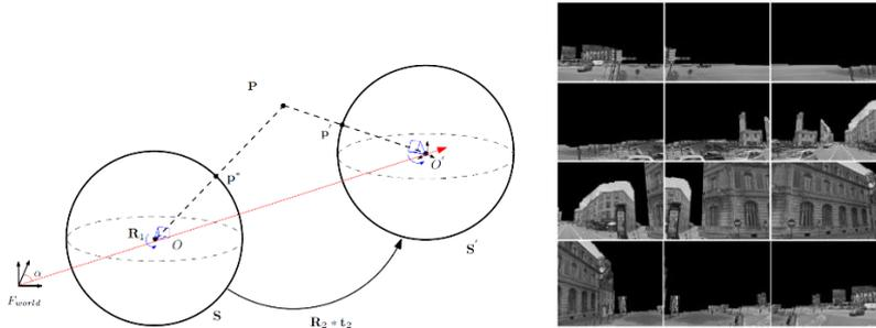
**Fig. 3.** Generation of rectilinear images from virtual viewpoints located in point  $O'$  translated from the centre  $O$  of the initial panorama. Black regions correspond to pixels for which the back-projection lies outside the original panorama, and is therefore unknown.
