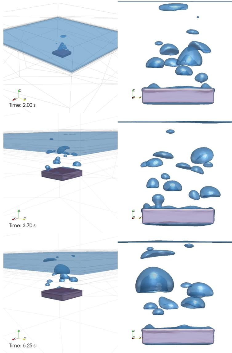
Figure 21: Industrial quenching. Results at  $t=2, 3.70$  et  $6.25$  s. Perspective view (left), front view (right). The zero isovalue of the level set is represented in blue.
