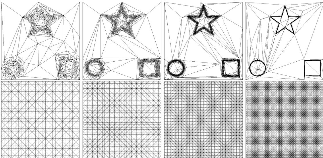
Figure 5: The obtained mesh for 1,000, 2,000, 5,000 and 10,000 elements.
