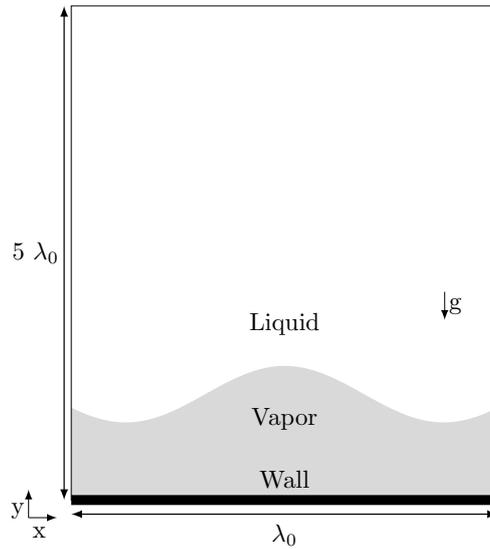
Figure 10: Setup for the 2D film boiling
