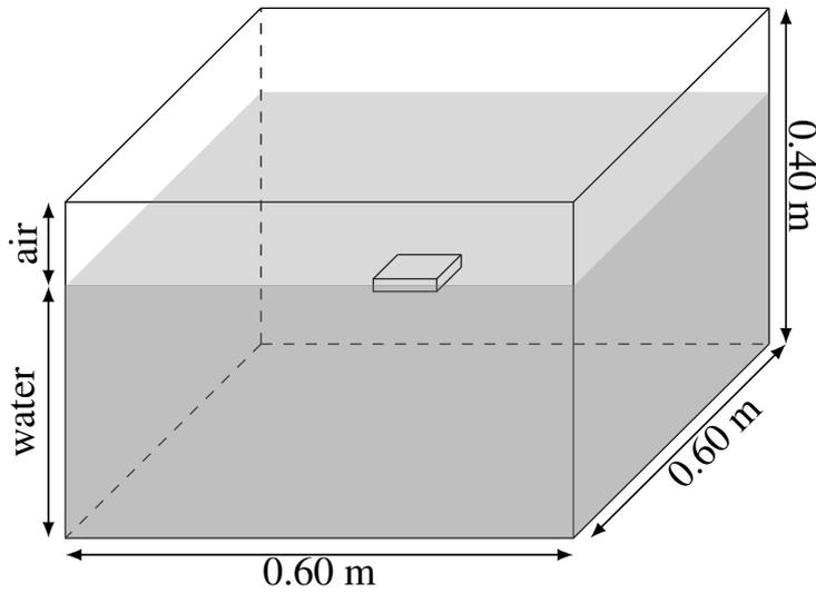
Figure 20: Set-up for the 3D industrial quenching
