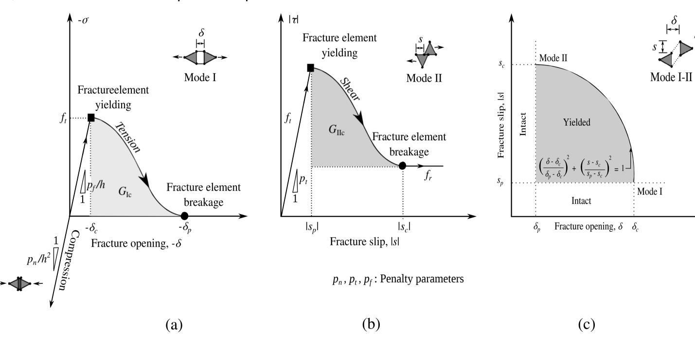
Figure 1: Penalty coefficients and fracture energies for different modes of fracturing adopted in FDEM [1].
