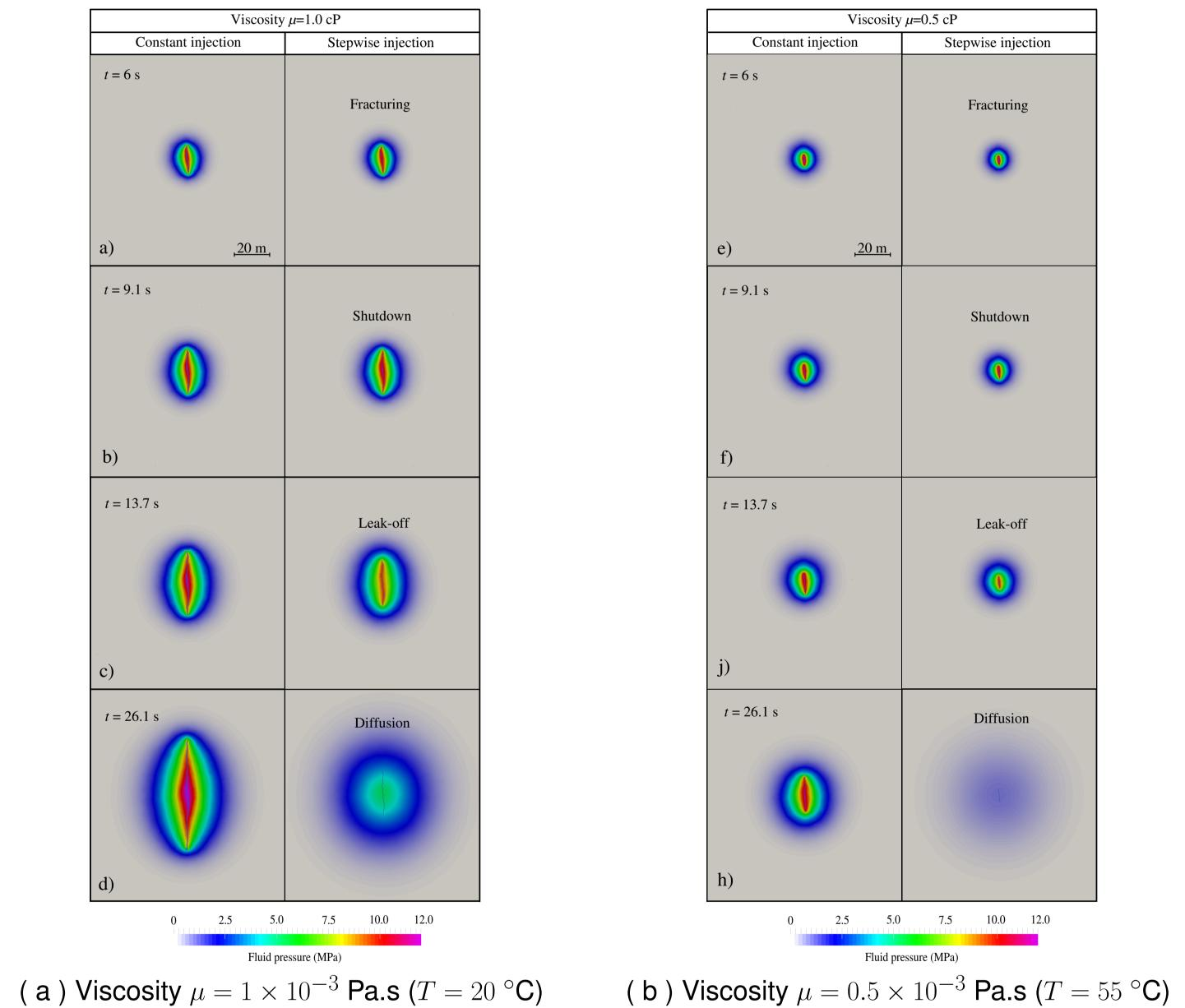
**Figure 8:** Fluid driven fracture patterns and diffused fluid pressure contours for the two schemes of injection and for tow different values of fluid viscosity, i.e.  $\mu = 1 \times 10^{-3}$  Pa.s corresponding to T = 20 °C and  $\mu = 0.5 \times 10^{-3}$  Pa.s corresponding to T = 55 °C. These contours and fracture patterns are plotted for several injection times which correspond to the letters (a to h) in Fig. 7.
