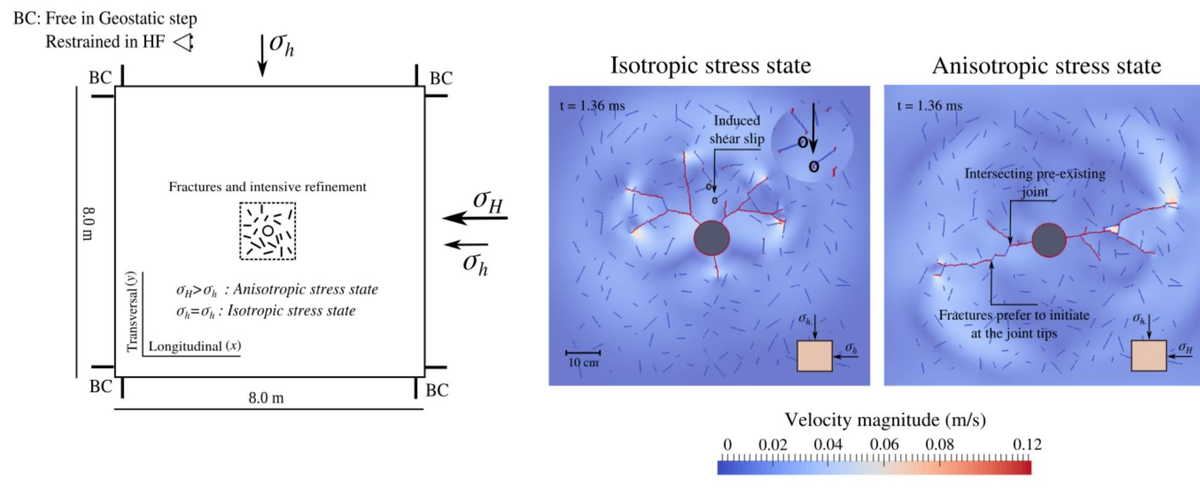
Figure 3: a) The model of the simulations used in the Y-Geo code. b) Fracture patterns for the cases of isotropic and anisotropic stress states in a heavily fractured rock formation at time of 1.36 ms since injection. The trajectories are plotted in the field of velocity magnitude.
