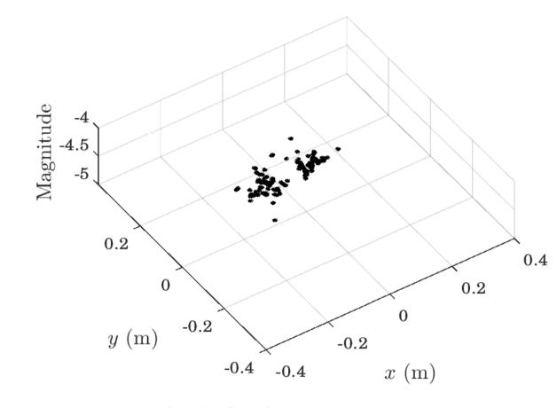
( a ) At time 1.28 ms Figure 5: Magnitudes of the microseismic events presented in Fig. 4. The values are in the range of monitored HF induced microseismicity.
