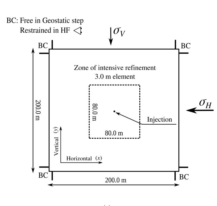
Figure 6: (a) The geometry and boundary conditions of domain chosen for the HF simulations (Irazu code).
