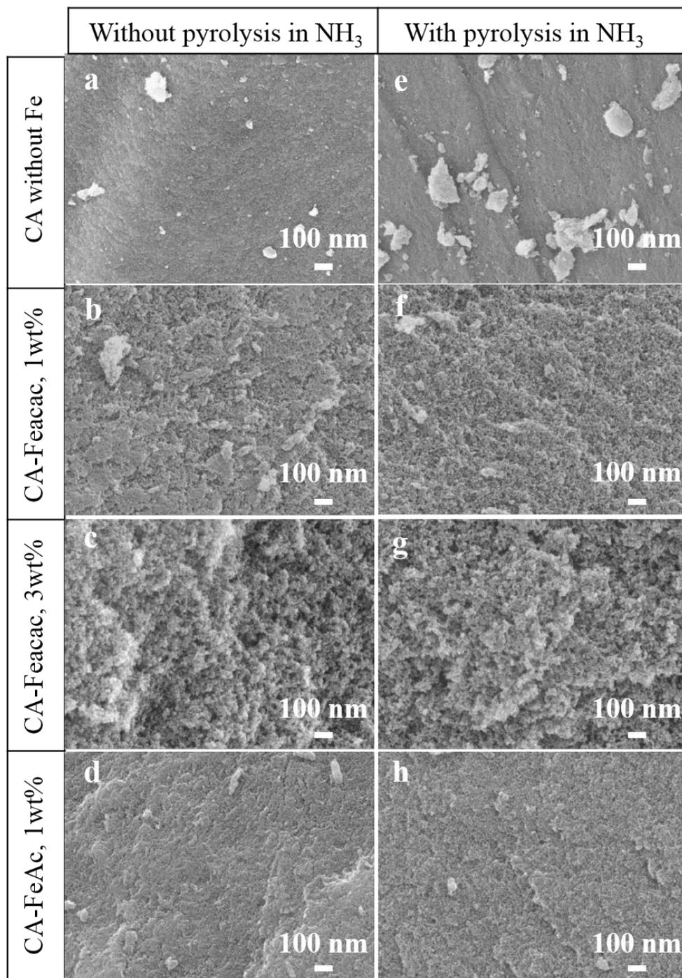
Fig. 2 SEM of catalysts with and without pyrolysis in NH<sub>3</sub> for carbon aerogels without Fe (a and e), with 1wt% of Fe using Feacac precursor (b and f), with 3wt% of Fe using Feacac precursor (c and g) and with 1wt% of Fe using FeAc precursor (d and h).
