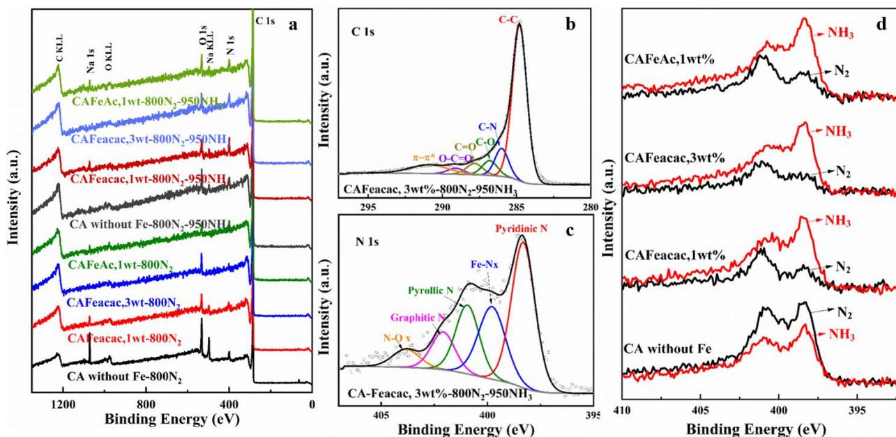
Fig. 5 XPS spectra and analyses of aerogel catalyst. Survey scans (a); High-resolution (HR) XPS spectra of C 1s (b) and N 1s (c) for CA-Feacac, 3wt%-800N<sub>2</sub>-950NH<sub>3</sub>; The comparison of N 1s (d) spectra prepared under different conditions.
