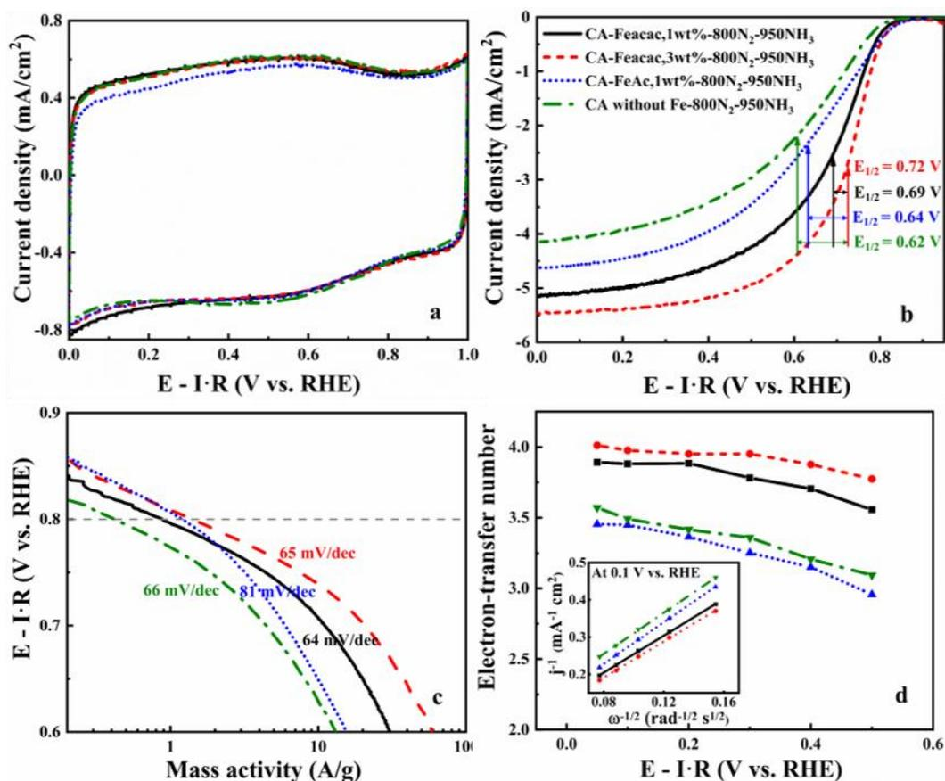
Fig. 6 CVs in 0.05 M H<sub>2</sub>SO<sub>4</sub> deaerated solution with a potential scan rate of 10 mV s<sup>-1</sup> (a), polarization curves in RDE at 1600 rpm at 10 mV s<sup>-1</sup> O<sub>2</sub>-saturated 0.05 M H<sub>2</sub>SO<sub>4</sub> (b), tafel plots (c) and Electron-transfer number (d) over 0.05-0.7 V of catalysts. Inset of Fig. 6d: The K-L plot at 0.1 V vs. RHE.
