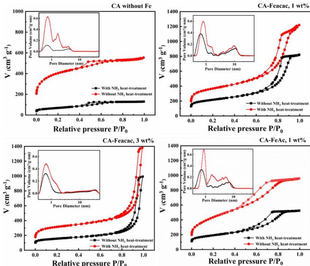
Fig. 3  $N_2$  adsorption isotherms at 77 K of the Fe-N-C aerogels pyrolyzed at 800 °C in  $N_2$  with and without HT in  $NH_3$ . Inset: Pore size distribution plots obtained by using the 2D-NLDFT-HS method.
