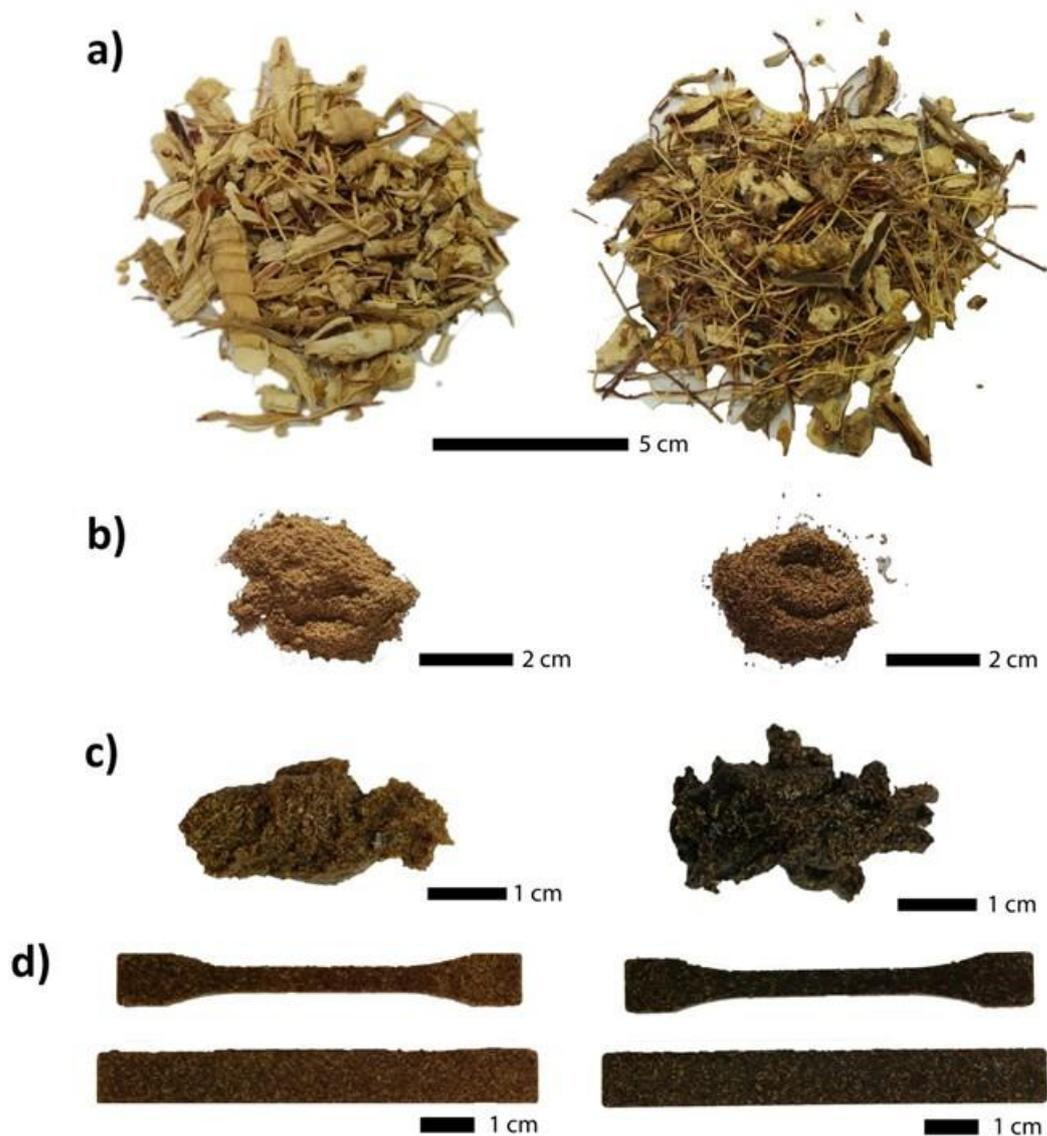
**Figure 1.** Physical aspect of GIG (left) and GOL (right) belowground materials a) before grinding, b) after sieving (fraction collected with 200-300  $\mu\text{m}$  openings), c) after mixing in the internal mixer, and d) after injection molding.
