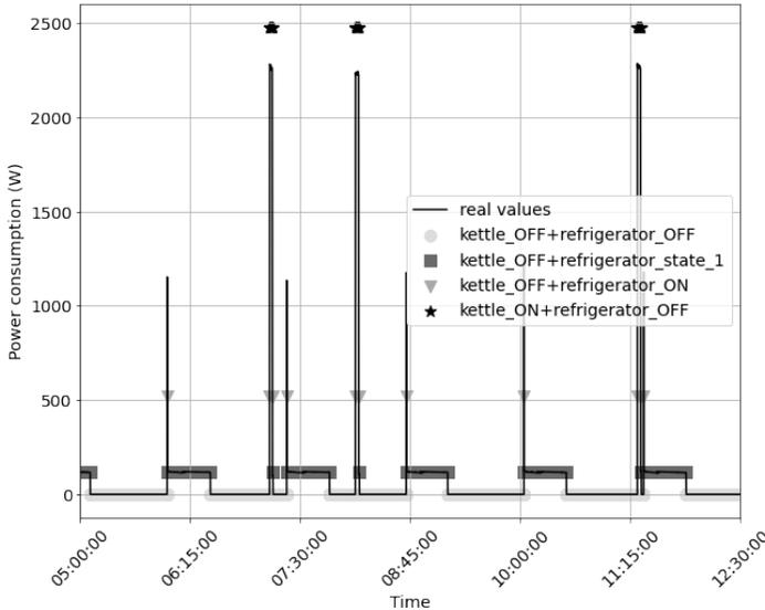
Fig. 1. States predictions HMM of hot-water boiler and refrigerator combined, sampling rate = 1 second
