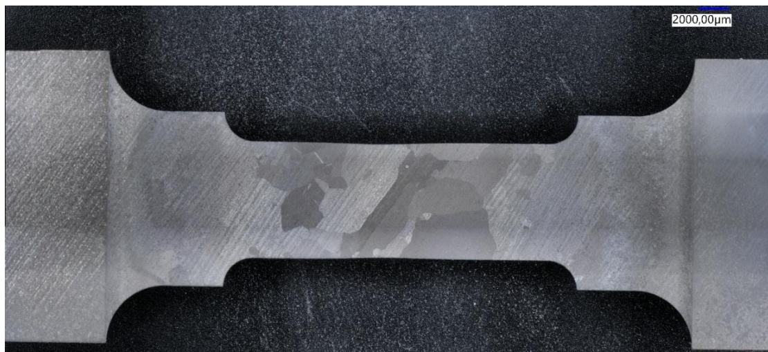
Figure 4. \langle 111 \rangle specimen after non-isothermal loading up to 9600 N, standard homogenization heat treatment and subsequent etching.
