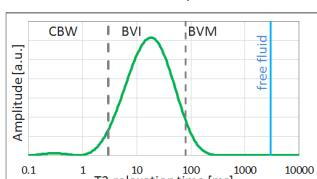
Fig 2: T<sub>2</sub> distribution of a set of cuttings without external fluid
