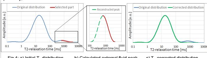
If cuttings are oversaturated, the corrected NMR porosity is lower than the NMR porosity, but if cuttings are undersaturated, both values are equal.
