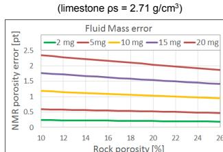
Fig 1: NMR porosity error as a function of the fluid mass error
