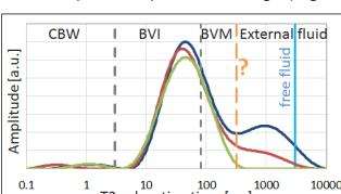
Fig 3: T<sub>2</sub> distribution of sets of cuttings with decreasing amounts of external fluid
