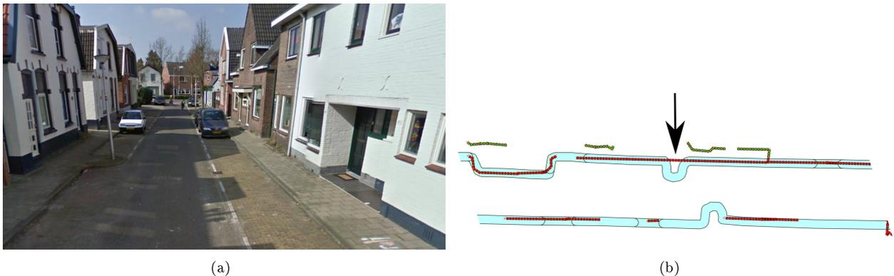
Figure 4.19: Inconsistent ground truth lines on *Enschede* dataset. Ground truth (cyan) presents an extrusion that does not correspond to the real curb. Detected curbs (red) and building entrances (green). Photo taken from Google Street View, taken another day, so parked cars are not the same.
