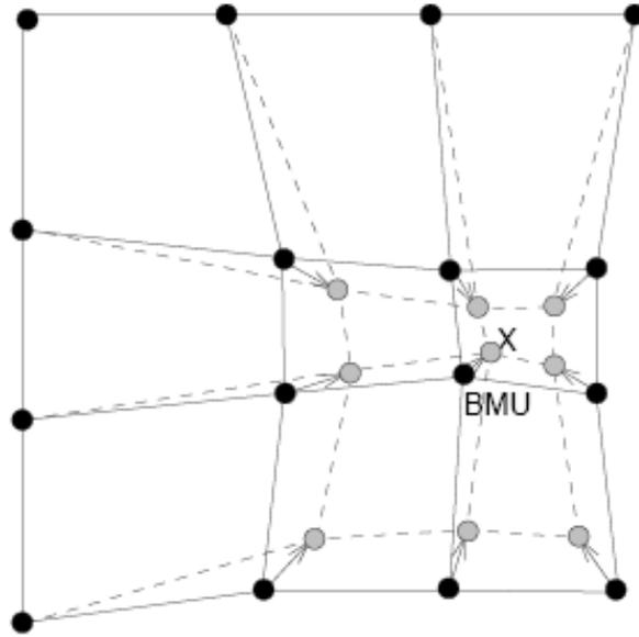
Figure 3.2: Scheme of competitive training of self-organizing neural networks.  $X$  represents a 3D point of the input point cloud, and BMU is the closest neuron to  $X$ , called the best match unit. Note that the BMU neighbors are adapted iteratively.
