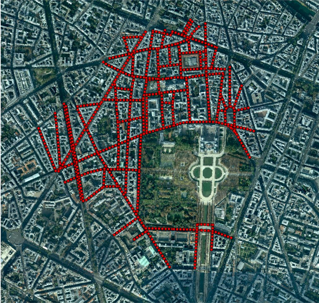
Figure 4.10: Road medial axes in the 6<sup>th</sup> Parisian district. Information available from IGN France. This information is used in order to avoid false curb reconnections crossing the road, only reconnections on the same city block are allowed.
