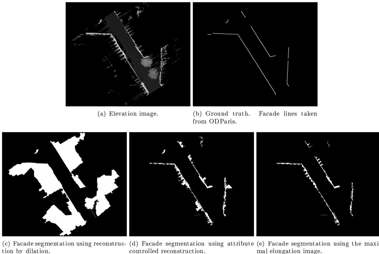
Figure 5.21: Facade segmentation results for site II (TerMob2\_LAMB93\_0021.ply). (a) presents the elevation image, (b) the GT annotations and (c,d,e) the segmentation results using our three proposed methods.
