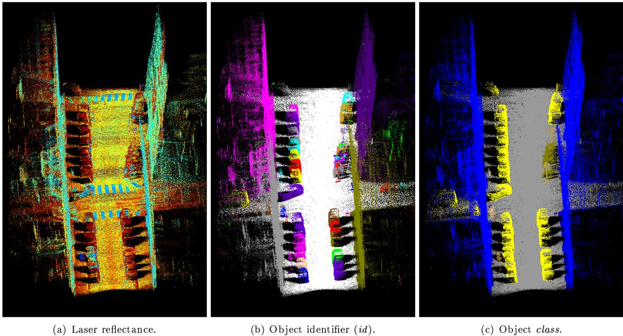
Figure 2.8: Paris-rue-Madame dataset: “GT\_Madame1\_2.ply” manually annotated file. 3D point cloud colored by its available fields. For object id: each color represents a different object (some colors may look similar when displaying). For object class: facades (blue), ground (gray), cars (yellow), motorcycles (olive), traffic signs (goldenrod), pedestrians (pink).
