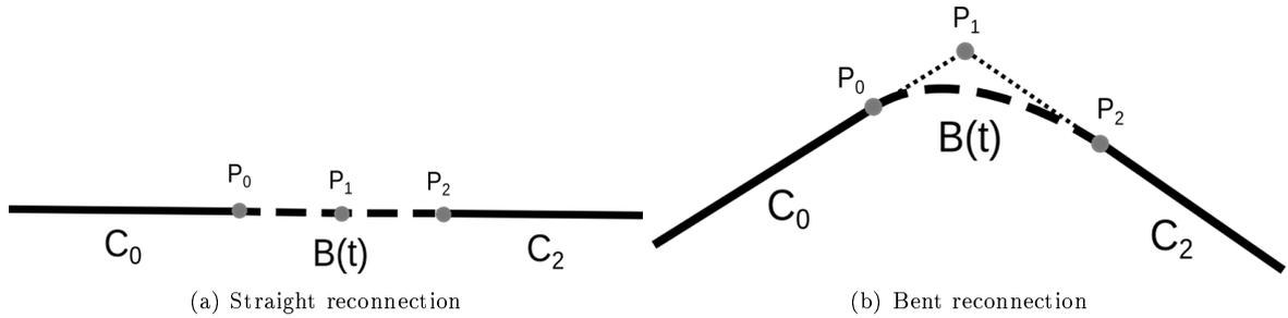
Figure 4.7: Quadratic Bézier reconnection in straight and bent cases. (a) if the curbs to be reconnected are co-linear,  $P_1$  is put in the middle of the segment  $\overline{P_0P_2}$ . Therefore, the resulting reconnection is a straight line. (b) if the curbs to be reconnected are not co-linear,  $P_1$  is put in the intersection of the two projection lines from  $C_0$  and  $C_2$ . Therefore, the resulting reconnection is a parabolic segment.
