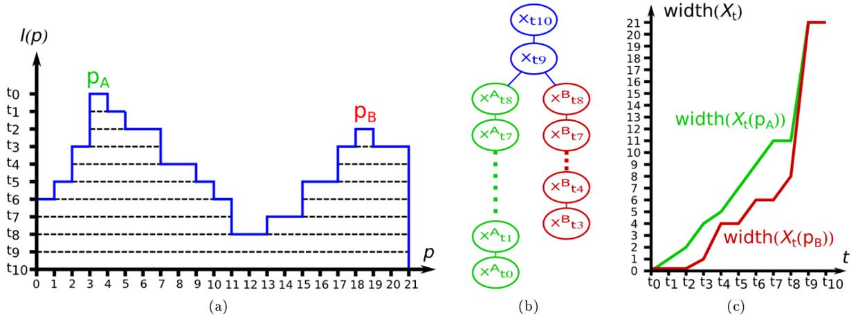
Figure 5.12: (a) 1D threshold decomposition; (b) component tree; (c) attribute (width) profile for the two maxima ( $p_A$  and  $p_B$ ). Events on this attribute profile are useful to segment objects, extract features and define adaptive structuring elements.
