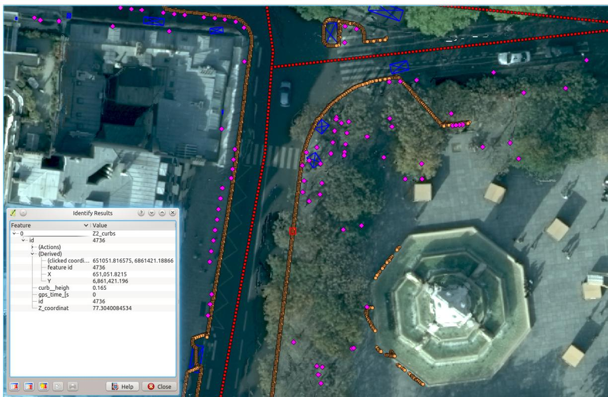
Figure 4.15: Obstacle map and accessibility information exported into a GIS. Curbs (orange), bollards (magenta), medial road axes (red), obstacle bounding box (blue).
