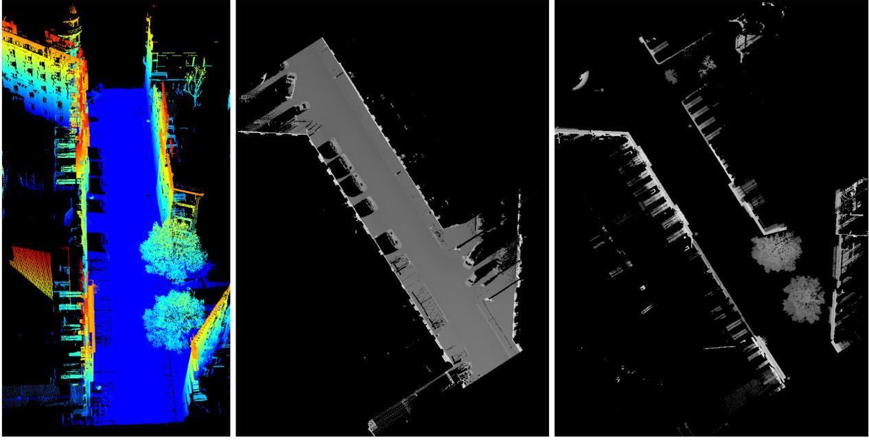
(a) 3D point cloud colored by the Z coordinate. (b) Elevation image from the lower slice: points between the ground level and  $H_{\text{slice}}$ . (c) Elevation image from the upper slice: points higher than  $H_{\text{slice}}$ .
