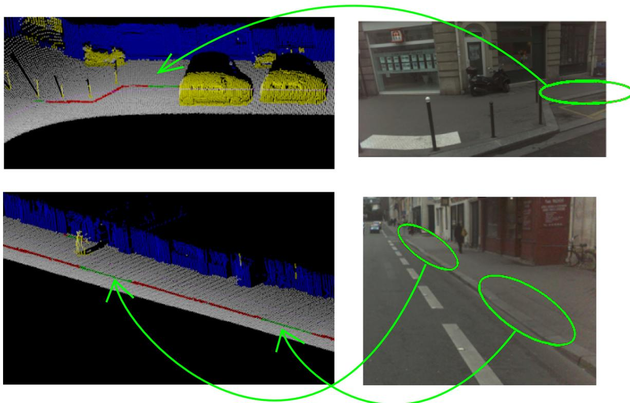
Figure 4.13: Curbs accessibility on two test sites in *rue Cassette* and *rue Vaugirard* in Paris, respectively. 3D labeled point clouds: facades (blue), urban objects (yellow), ground (gray), inaccessible curb (red), accessible curb (green). Acquisition by IGN©France.
