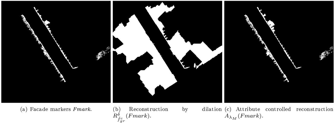
Figure 5.9: Comparison of facade segmentation methods using reconstruction by dilation and attribute controlled reconstruction on the ground residue image. Test site in *rue d'Assas* in Paris, France. Stereopolis II, IGN©.
