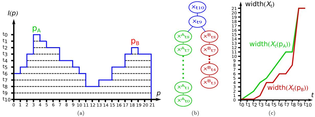
Figure 7.2: (a) 1D threshold decomposition; (b) component tree; (c) attribute profile for a 1D function from its two maxima ( $p_A$  and  $p_B$ ). Events on this attribute profile are useful to segment objects (Jones, 1999), extract features (Pesaresi and Benediktsson, 2001; Beucher, 2007; Morard et al., 2011b) and define adaptive structuring elements (Serna and Marcotegui, 2013a).
