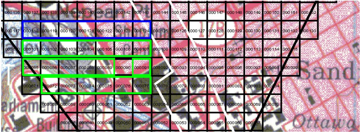
Figure 6.21: Ottawa city, Ohio (USA). The database contains 26 annotated tiles  $100 \times 100$  meters each. A typical scene contains trees, cars, lampposts, among others. The GT consists in a labeled point marking the center of each object and its class. This database contains three types of tiles: training (blue), test (green) and non-annotated (black).
