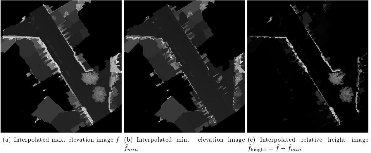
Figure 5.2: Interpolated elevation images from a test site in *rue d'Assas* in Paris, France. (a) and (b) show interpolated maximal  $\hat{f}$  and interpolated minimal  $\hat{f}_{\text{min}}$  elevation images, respectively. Note that interpolated relative height image  $\hat{f}_{\text{height}}$  is appropriate to compute facade markers since it contains information about high and vertical urban structures, as shown in (c). Acquired by Stereopolis II, IGN©.
