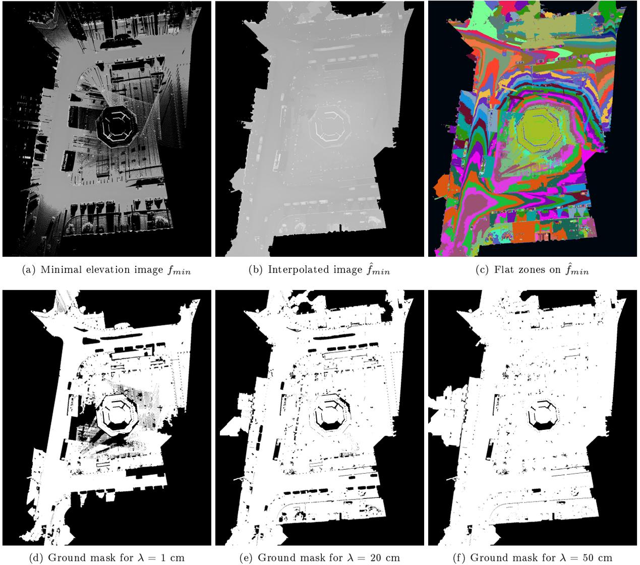
Figure 4.3: Ground segmentation: extraction of the largest quasi-flat (called also  $\lambda$ -flat) zone on interpolated minimal elevation image  $\hat{f}_{min}$ . The  $\lambda$  parameter chosen for our experiments is 20 cm. Test site in *St. Sulpice* square in Paris, France. Stereopolis II, IGN©.
