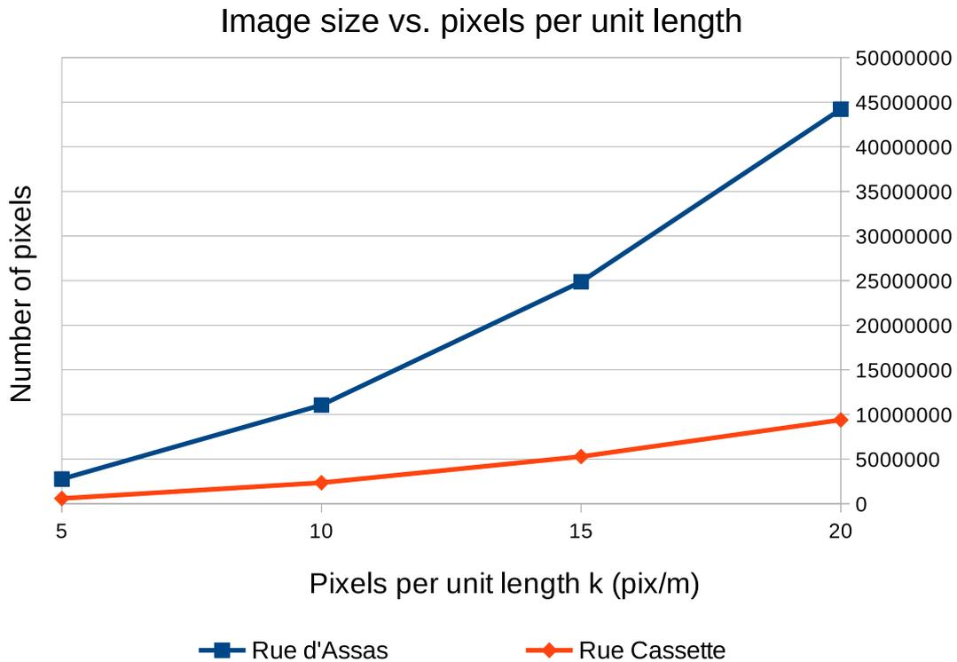
Figure 3.9: Elevation image size for different  $k$  parameters (number of pixels per length unit) from 5 pix/m to 20 pix/m. The elevation image size has a critical effect in the computation time: the bigger the image, the slower the computation. It is noteworthy that the number of pixels increases as  $k^2$ .
