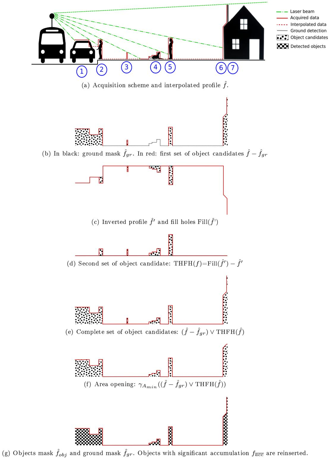
Figure 6.3: Detection method on a 1D profile. This urban scenario contains the following objects: ① car, ② pedestrian, ③ noisy structure, ④ dog, ⑤ pedestrian, ⑥ house facade, and ⑦ chimney.
