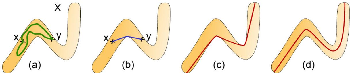
Figure 7.3: Geodesic diameter  $L(X)$  definition. (a) Two paths between points  $x$  and  $y$ ; (b) geodesic arc between these two points; (c) longest geodesic arc of object  $X$ , whose length is the geodesic diameter  $L(X)$ ; (d) generalized geodesic distance, longest geodesic arc. Image taken from Morard et al. (2013)
