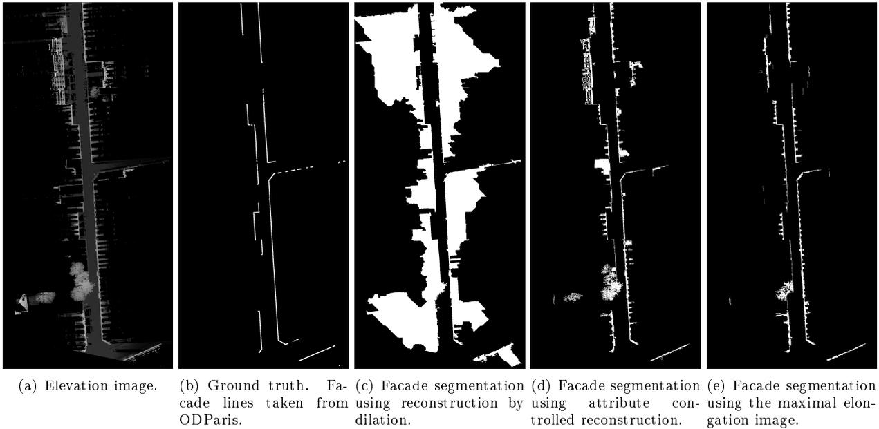
Figure 5.22: Facade segmentation results for site III (Cassette\_idclass.ply). (a) presents the elevation image, (b) the GT annotations and (c,d,e) the segmentation results using our three proposed methods.
