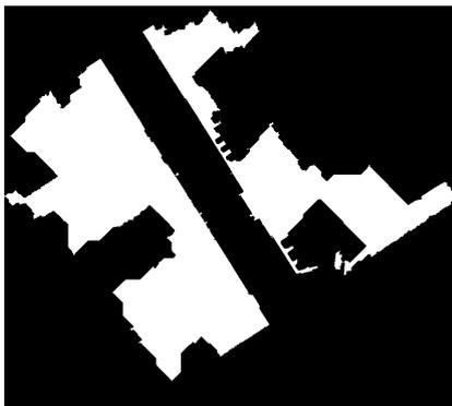
(c) Facade segmentation using reconstruction by dilation.
