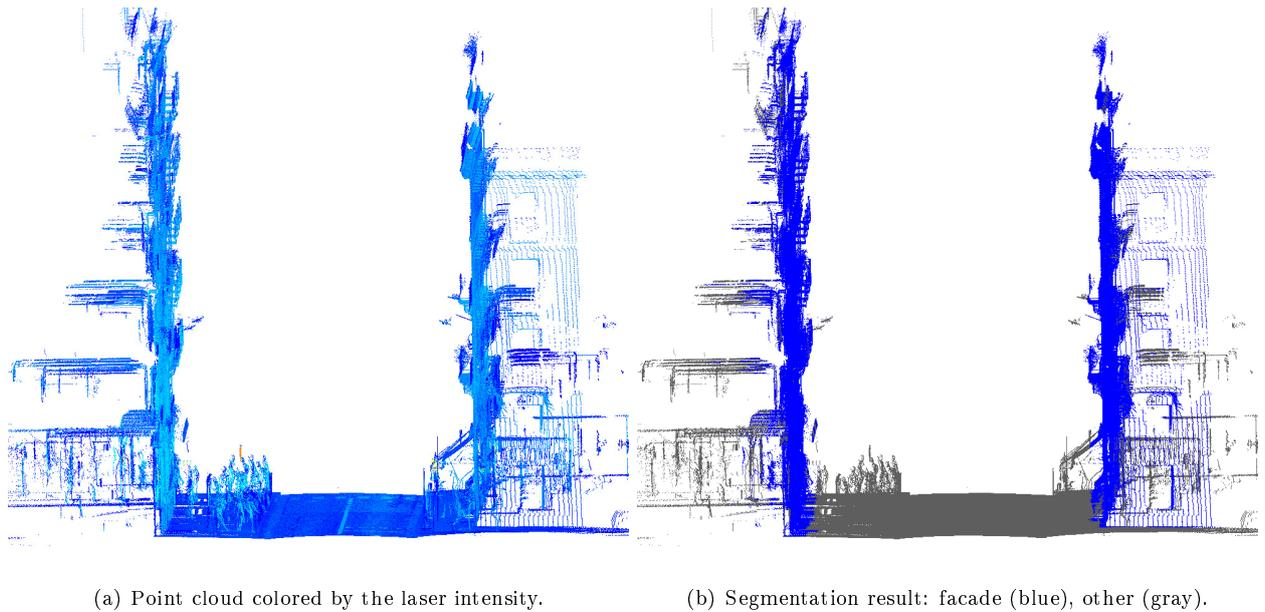
Figure 5.10: Facade segmentation using attribute controlled reconstruction on the ground residue image. Note that using this attribute controlled reconstruction, the store, the pedestrians and the traffic sign have been correctly separated from the facade. Test site in *rue d'Assas* in Paris, France. Stereopolis II, IGN©.
