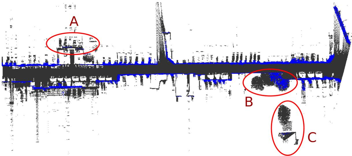
Figure 5.24: Facade segmentation result using the maximal elongation image on “Cassette\_idclass.ply” file. Ground (gray), facades (blue). Input file taken from TerraMobilita/iQmulus database. Stereopolis II, IGN©. Errors are due to an incomplete detected facade (zone A) and a tree alignment connected to a low wall (zone B). Zone C corresponds to non-annotated points.
