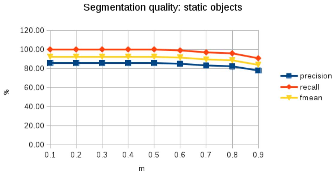
Figure 6.18: Segmentation quality for *static object* class on the TerraMobilita/iQmulus database. The geometric quality of our segmentation is good since the performance decays slowly. For example,  $f_{\text{mean}}(m)$  decays from 87.80 % to 78.05 % for  $m$  varying from 0.1 to 0.9. Note that in the range  $m=[0.1, 0.5]$  our performances are constant, while in the range  $m=[0.5, 0.9]$  the  $f_{\text{mean}}(m)$  decays less than 10%, proving the robustness of our segmentation approach.
