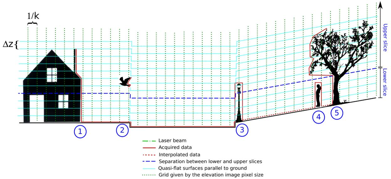
Figure 6.11: Adaptive voxelization using quasi-flat surfaces parallel to the ground. This example contains five objects: ① facade, ② bird, ③ lamppost, ④ pedestrian, and ⑤ tree. Using such structure, 3D connectivity can be defined using 6- or 26-neighborhoods.
