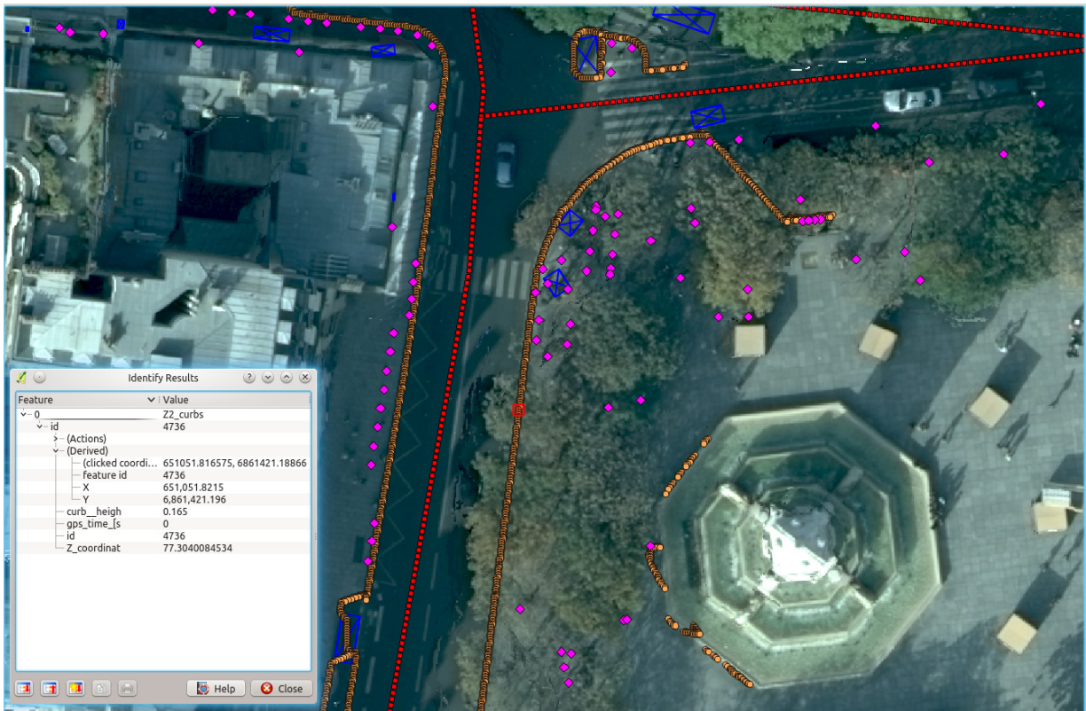
Figure 4.15: Obstacle map and accessibility information exported into a GIS. Curbs (orange), bollards (magenta), medial road axes (red), obstacle bounding box (blue).
