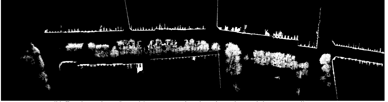
(b) Facade markers. Several incorrect markers have been detected due to tree alignments.
