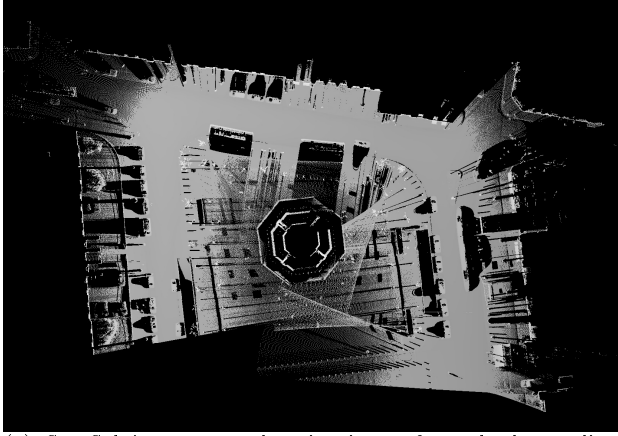
(a) St. Sulpice square: elevation image from the lower slice: points between the ground level and H_{\text{slice}} .
