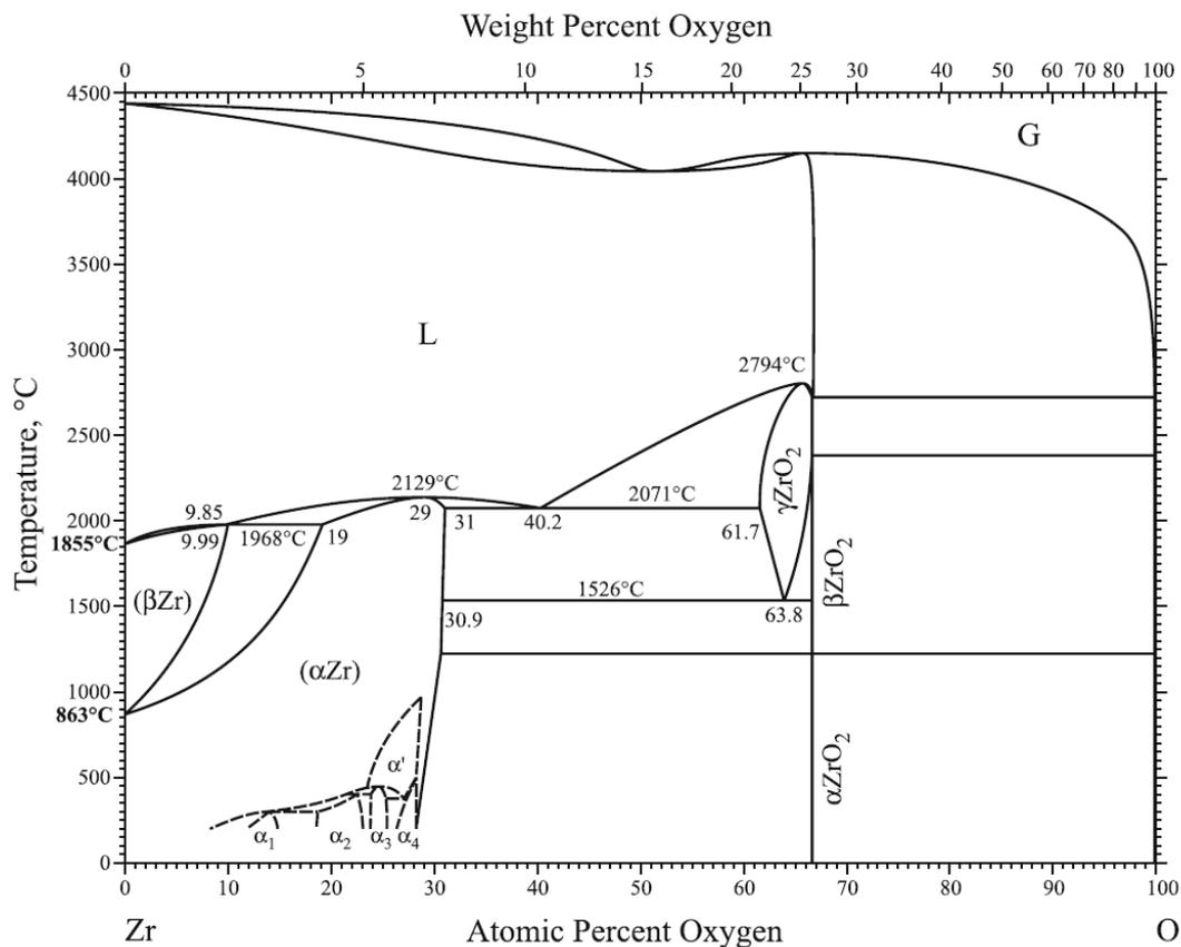
FIGURE I.12 – Diagramme de phases binaire Zr – O [58].
